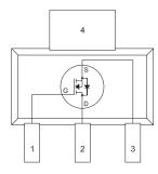
Tab is common to pin 2 (Top View)
