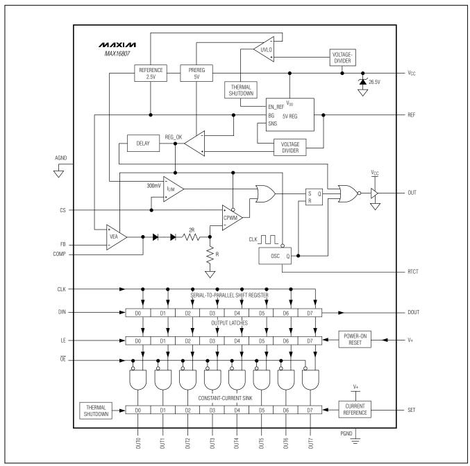
Figure 1a. Internal Block Diagram (MAX16807)
