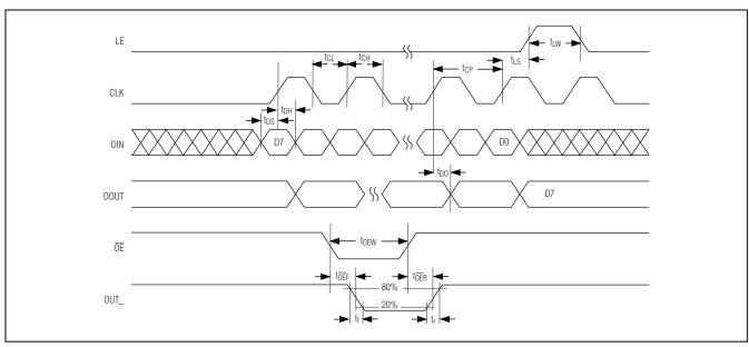
Figure 3. 4-Wire Serial-Interface Timing Diagram
