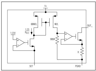
Figure 1c. OUT\_ Driver Internal Diagram
