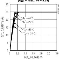
OUT\_ CURRENT vs. OUT\_ VOLTAGE (R<sub>SET</sub> = 720 $\Omega$ , V+ = 5.0V)
