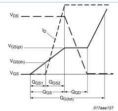
Fig. 16. Gate charge waveform definitions
