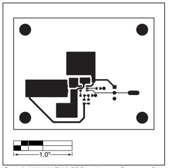
Figure 3. MAX1896 EV Kit PC Board Layout—Component Side
