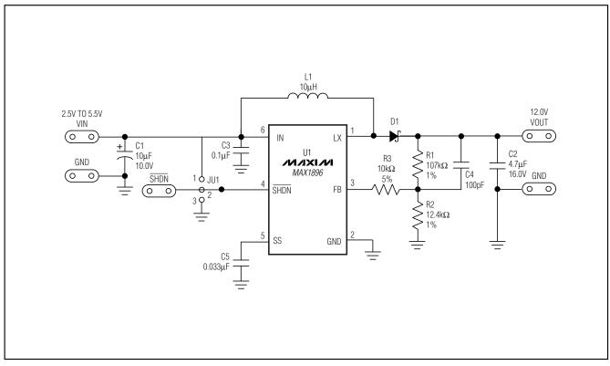
Figure 1. MAX1896 EV Kit Schematic
