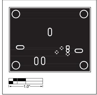
Figure 4. MAX1896 EV Kit PC Board Layout—Solder Side
