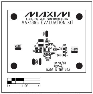
Figure 2. MAX1896 EV Kit Component Placement Guide—Component Side
