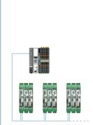
I/O to serial (Modbus RTU)
