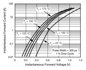
Fig. 3 - Typical Instantaneous Forward Characteristics
