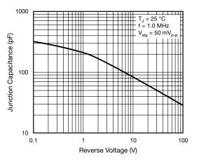
Fig. 5 - Typical Junction Capacitance
