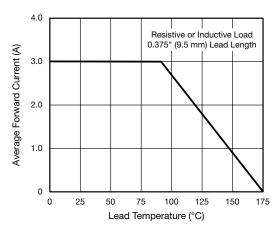
Fig. 1 - Forward Current Derating Curve
