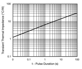
Fig. 6 - Typical Transient Thermal Impedance
