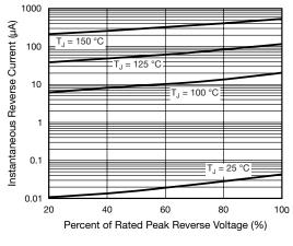
Fig. 4 - Typical Reverse Characteristics
