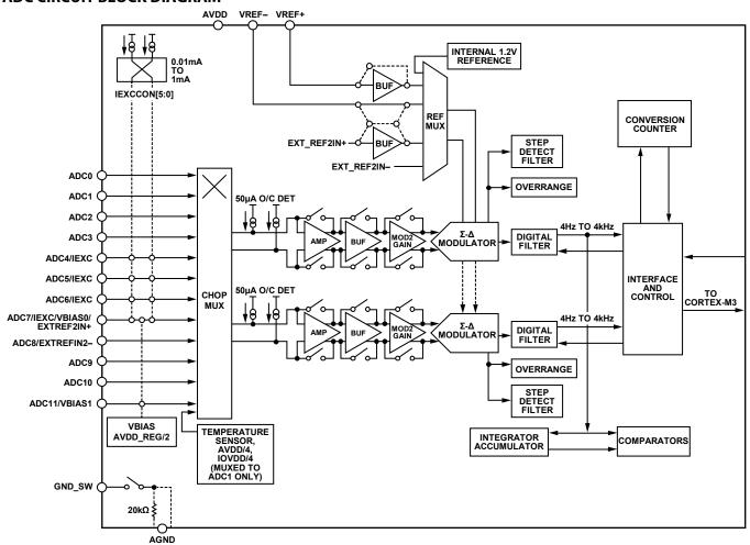
Figure 5. ADC Block Diagram
