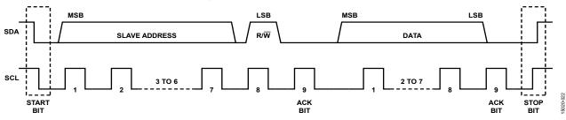
Figure 23. Typical I<sup>2</sup>C Transfer Sequence
