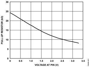
Figure 22. GPIO Pull-Up Resistor Value
