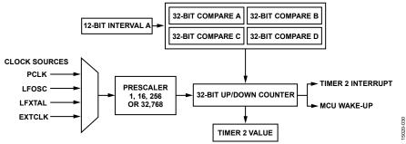
Figure 32. Wake-Up Timer Block Diagram
