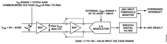
Figure 6. ADC Inputs
