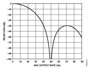
Figure 15. Digital Filter Frequency Response, Notch 2 Filter Off
