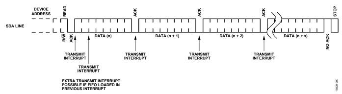
Figure 26. I<sup>2</sup>C Slave Tx Interrupt Details
