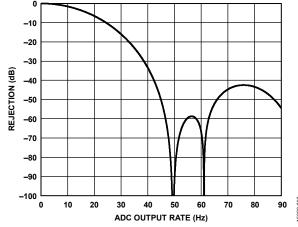
Figure 14. Digital Filter Frequency Response, Notch 2 Filter On
