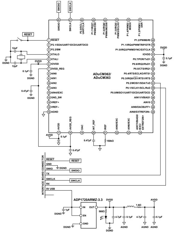
Figure 40. Typical System Configuration
