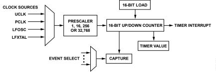
Figure 31. General-Purpose Timers Block Diagram
