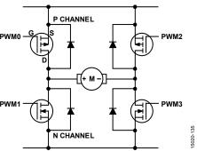
Figure 37. Example H-Bridge Configuration
