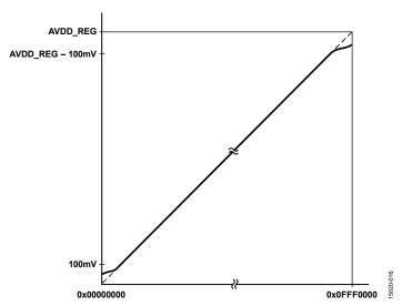
Figure 17. DAC Endpoint Nonlinearities Due to Amplifier Saturation
