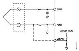
Figure 11. Using V<sub>BIAS</sub> Voltage to Set Thermocouple Common-Mode Voltage
