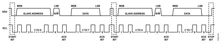
Figure 25. I<sup>2</sup>C Repeated Start Sequence
