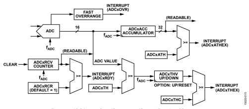
Figure 16. ADC Accumulator/Comparator/Counter Functional Diagram
