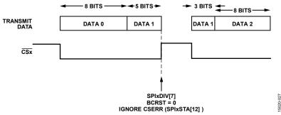
Figure 29. SPI Communication: Midbyte Stall
