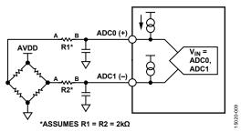
Figure 10. Example Circuit Using Diagnostic Current Sources
