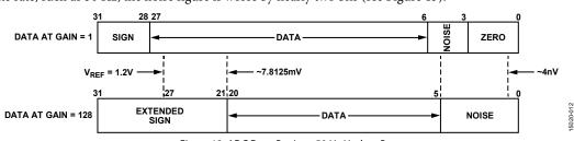
Figure 13. ADC Data Register 50 Hz Update Rate
