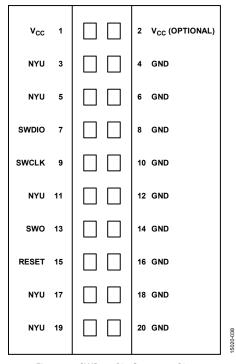
Figure 41. SWD 20-Pin Connector Pinout
