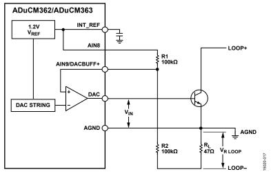
Figure 18. DAC NPN Mode: Typical Operation
