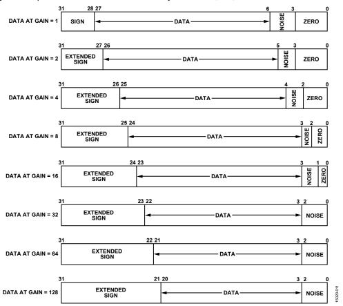
Figure 12. ADC Data Register 3.53 Hz Update Rate
