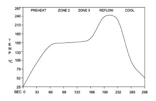
Fig. 3 Solder Reflow Temperature Profile
