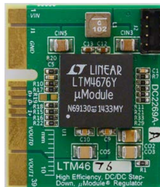
Figure 1. Dual-Output LTM4676/DC2269A-A Demo Circuit
