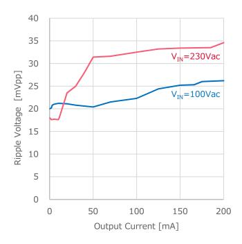
Figure 14. VOUT Ripple Voltage (I<sub>OUT</sub> vs. V<sub>ripple</sub>)
