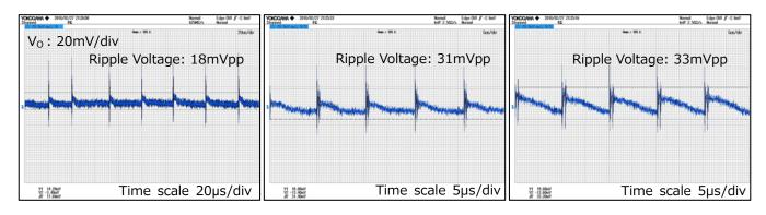
$V_{IN}$ =230Vac, IOUT=10mA Figure 18. VOUT Ripple Voltage.4  $V_{IN}$ =230Vac,  $I_{OUT}$ =50mA Figure 19. VOUT Ripple Voltage.5  $V_{IN}$ =230Vac,  $I_{OUT}$ =125mA Figure 20. VOUT Ripple Voltage.6
