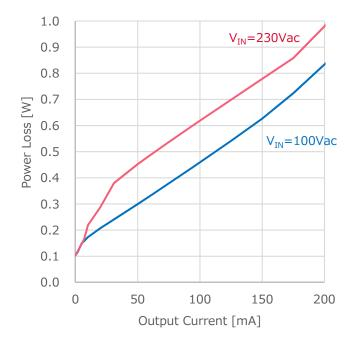
Figure 8. Load Regulation (I<sub>OUT</sub> vs. P<sub>LOSS</sub>)
