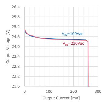
Figure 6. Load Regulation ( $I_{OUT}$  vs.  $V_{OUT}$ )
