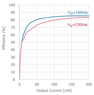
Figure 7. LOAD Regulation (I<sub>OUT</sub> vs. Efficiency)
