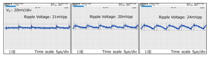
$V_{IN}$ =100Vac, IOUT=10mA Figure 15. VOUT Ripple Voltage.1
