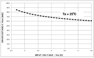
Fig.16 PMOS on resistance-power-supply voltage
