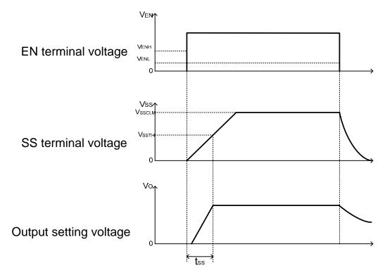
Fig.2 ON/OFF transition wave form in EN controlling
