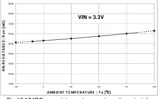
Fig.19 NMOS on resistance-temperature characteristic
