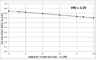
Fig.20 Terminal EN H voltage-temperature characteristic
