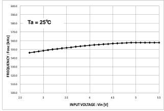
Fig.14 Switching frequency-power-supply voltage
