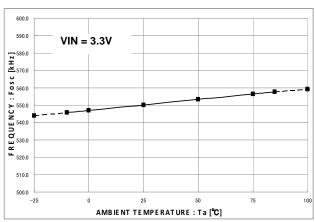
Fig.15 Switching frequency-temperature characteristic
