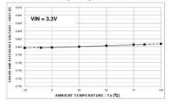
Fig.12 Reference voltage - Temperature characteristic
