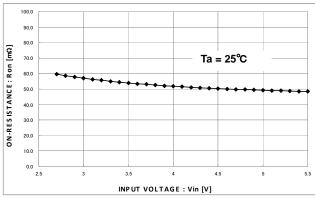
Fig.18 NMOS on resistance-power-supply voltage
