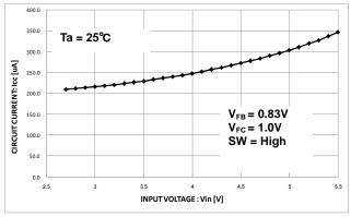
Fig.21 Circuit current-power-supply voltage characteristic
