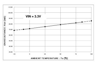
Fig.17 PMOS on resistance-temperature characteristic
