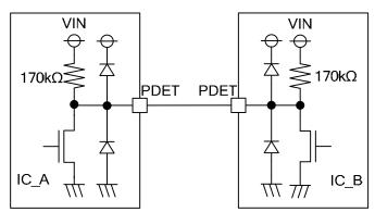
Fig.6 Protecting BUS communication
