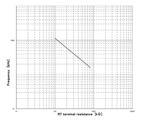
Fig.3 RT resistance-oscillation frequency
