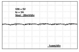
Fig.8 Output ripple
