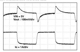
Fig.7 Output load response
