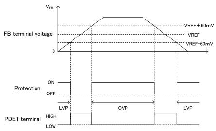
Fig.4 Output voltage error detection range
