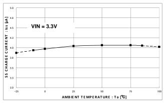
Fig.13 SS Charging current - Temperature characteristic
