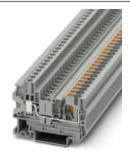
Feed-through terminal block, connection method: Push-in connection, Screw connection, cross section: 0.2 mm² - 6 mm², AWG: 24 - 12, width: 6.2 mm, color: black, mounting: NS 35/7,5, NS 35/15
