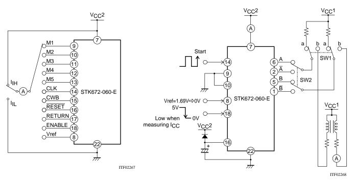
When measuring Ioave: With SW1 set to 'b', Vref = 1.69VWhen measuring fc: With SW1 set to 'a', Vref = 0VWhen measuring I<sub>CC</sub>: Set ENABLE low
