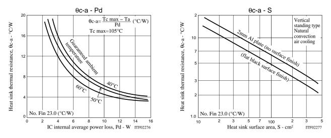
Next we determine the usage conditions with no heat sink by determining the allowable hybrid IC internal average loss from the thermal resistance of the hybrid IC substrate, namely 23°C/W.
