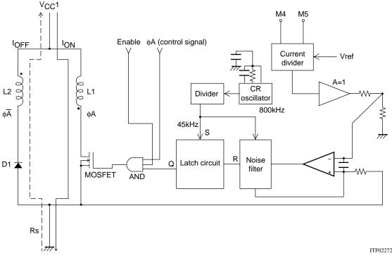
Driver Block Basic Circuit Structure
