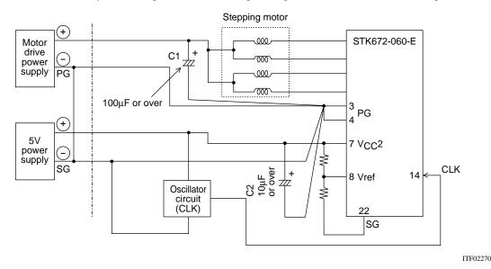
If the grounds for the motor drive supply and the hybrid IC 5V supply are separated:
