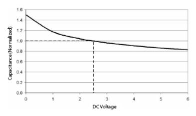
Figure 1. Diode Capacitance vs. Reverse Voltage
