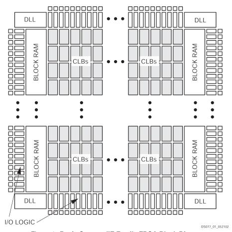
Figure 1: Basic Spartan-IIE Family FPGA Block Diagram
